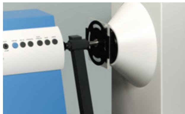
The measurement of haze is used to determine abrasion resistance of transparent materials. The Taber Abrasion Holder facilitates positioning of the abraded area in the measurement beam.
