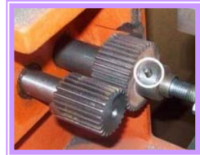
Adjusting Gear Equips W/ Inclined Safety Plug
